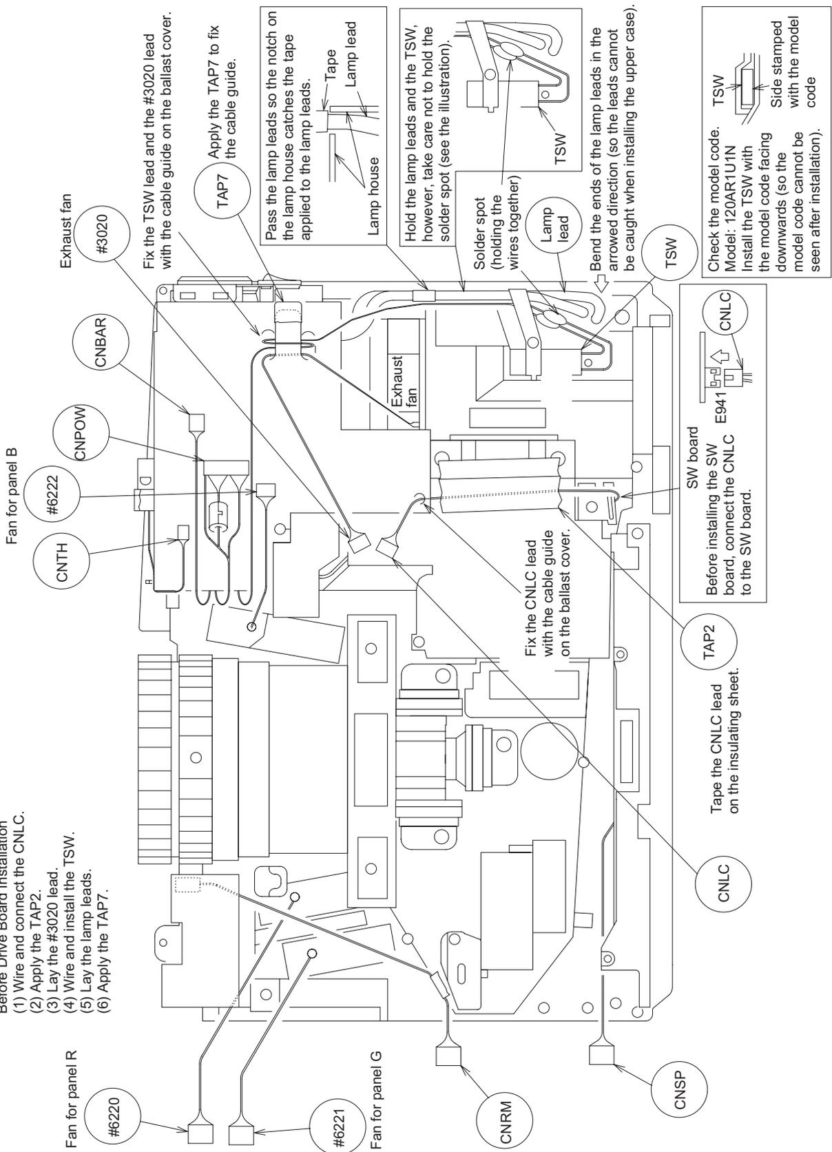
Wiring for Drive Board Installation
