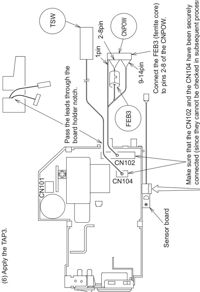
Install the sensor board after completing the following steps:
