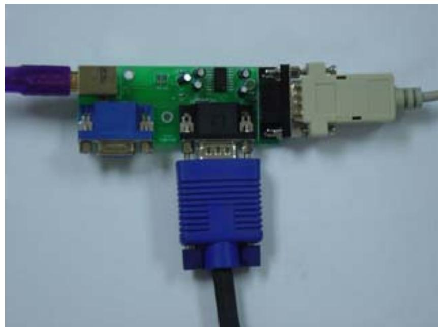
The 9-pin serial cable connects the com port of PC and the Genesis firmware update board. VP2330wb and the Genesis firmware update board is connected by VGA cable. The male A to male B USB cable connects the PC and Genesis firmware update board.
